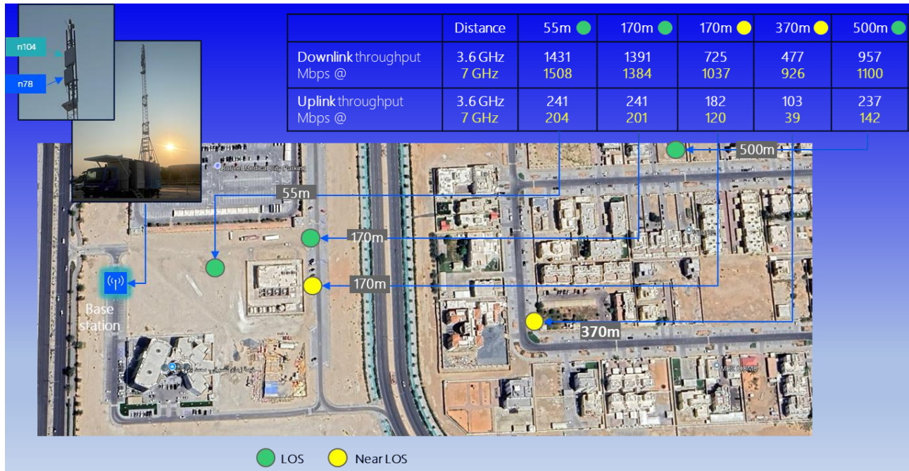
Figure 3. Field test measurement of UE from COW (cell on Wheel) site
