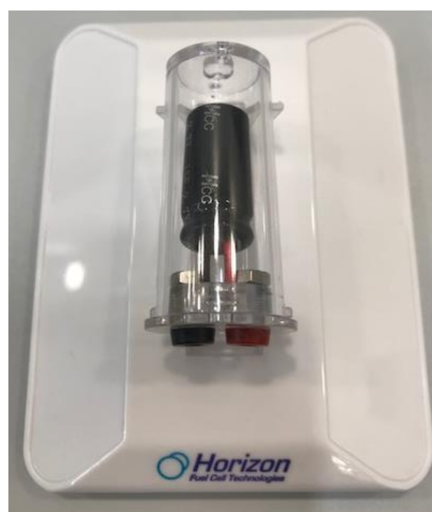
Supper Capacitor & its Stand
